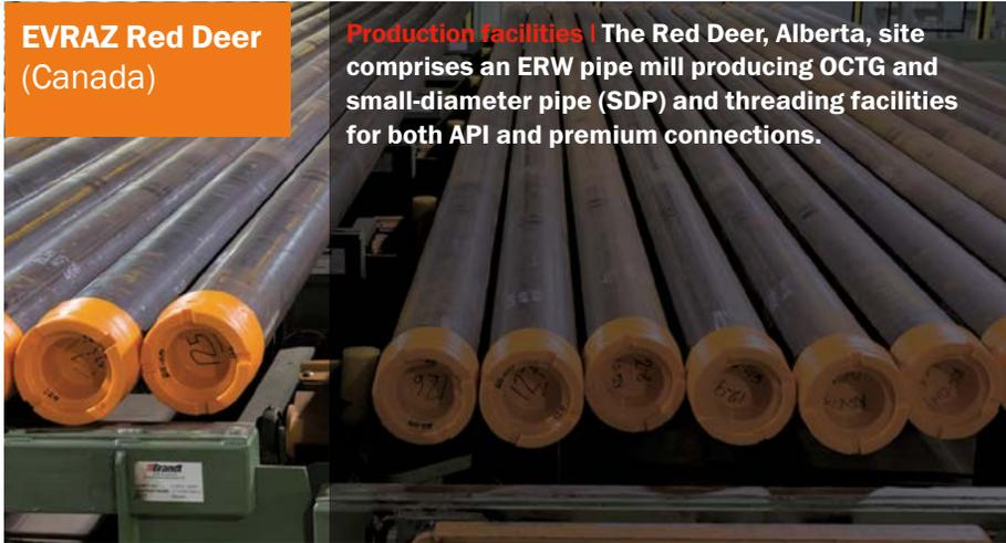
**Production facilities** | The Red Deer, Alberta, site comprises an ERW pipe mill producing OCTG and small-diameter pipe (SDP) and threading facilities for both API and premium connections.
